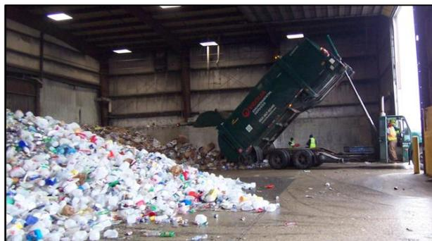
Recyclable materials delivered to the MRF tip floor.
